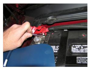
Removal of the battery and tray provides more room to get to the manifold bolts during a later step. Remove
